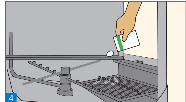
**Open delimer packet and drop 2 - 6 tablets into dishmachine depending on scale buildup**
