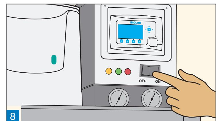
**Turn on tank heaters and carefully return detergent capsule to dispenser. For low-temperature machine, turn switch back to normal.**
