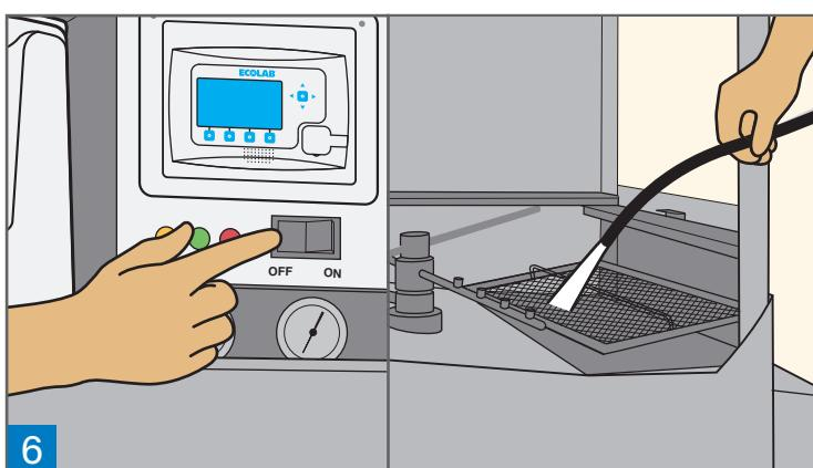
**Turn off machine and tank heater, drain and rinse inside machine thoroughly with fresh water.**
